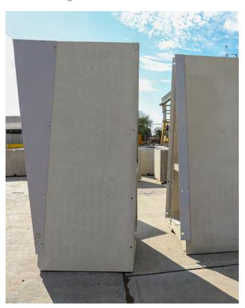
**7** If installing the Alfablocs against a solid vertical wall, then the strapless units should always be used to begin the installation of each new row of Alfablocs.
