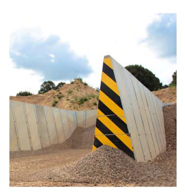
**18** The Alfablocs can be freestanding or alternatively bolted to the concrete by using threaded fixing bars. Extension tops can also be added to gain extra storage.
