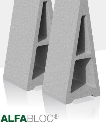
Alfabloc concrete security walling is the ideal solution for the protection of important infrastructure projects as well as traffic and crowd segregation. Alfabloc's patented jointed mechanism, utilising the use of steel interconnecting straps, creates a secure and substantial wall which can be erected quickly and easily.
